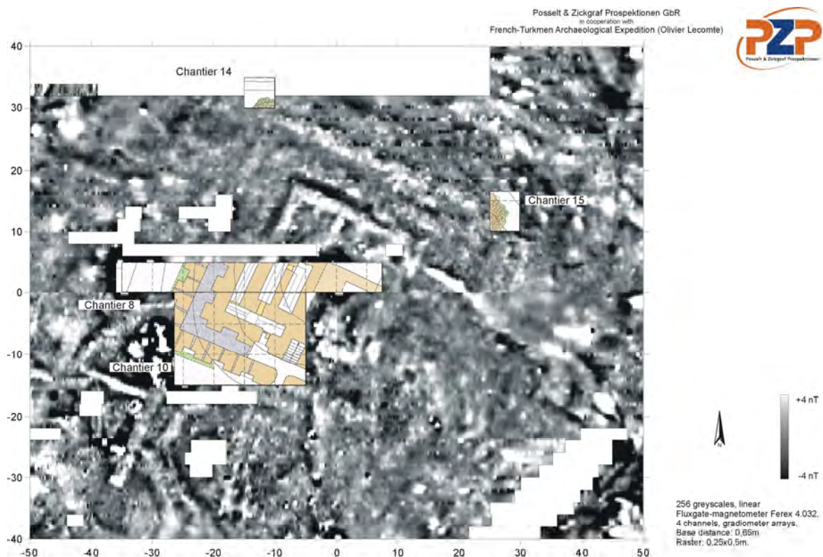
Fig. 12 Dushak, Etrap of Kaahka, Turkmenistan, "Ulug Depe". Geophysical survey 20-29 September 2003. Magnetometer survey. Excavation results (trenches 8,10,14-15) pasted to a detail of the magnetogram (excavation plots: French-Turkmen Archaeological Expedition). Slate: 24 May 2004.
